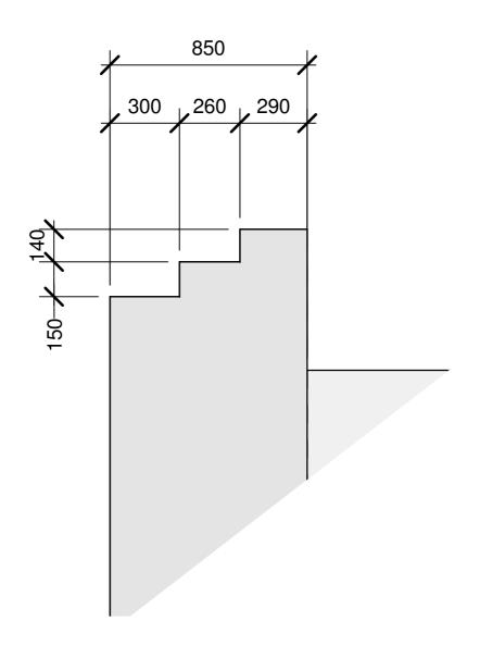
Abutment Detail Scale: 1:25
